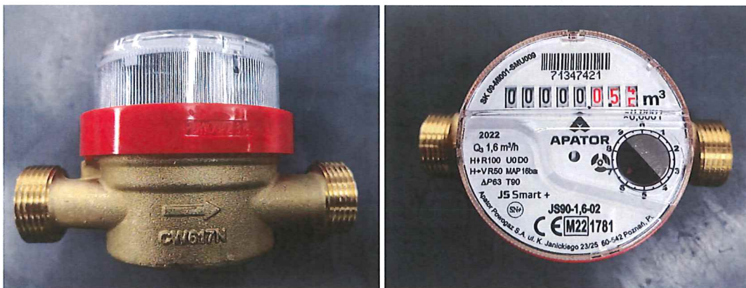
Picture No.1 Vane-wheel single-jet water meter JS90
