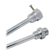
Installing thermostat series TH 140, place its head before securing the lock-nut. Do not rotate the thermostat head when lock-nut is secured as this can damage the thermostat.
