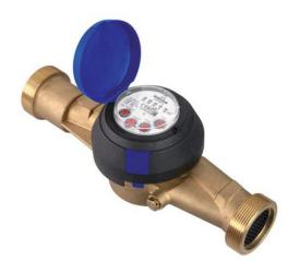
meters JS Master + are equipped with impulse transmitter (JSNK) or adapted for installation of the transmitter (JS-NKP), in standard version with five-barrel counter (IP65), brass housing, antimagnetic protection. Water meters are adapted to operation in the systems of remote data transfer (AMR).
