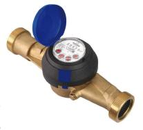
counter directed sidewards (V). Water meters JS Master c+ are equipped with impulse transmitter (JS-NK) or adapted for installation of the transmitter (JS-NKP), in standard version with five-barrel counter (IP65), brass housing with antimagnetic protection. Water meters are adapted to operation in the systems of remote data transfer (AMR).
