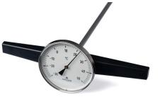
The thermometer consists of stainless steal head and stem made of galvanized steel tube. The end of the stem is terminated by smike of easier inserting into the measured medium and is provided with surface protection. Removable handle and fastening ring are parts of the thermometer.
